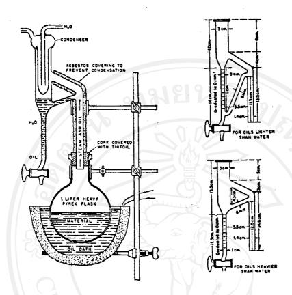
Figure 3: Volatile-oil distillation apparatus.
