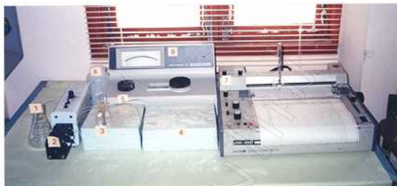
Figure 2.3 : reversed FIA system for the determination of Al(III) with tetracycline as a complexing agent.
