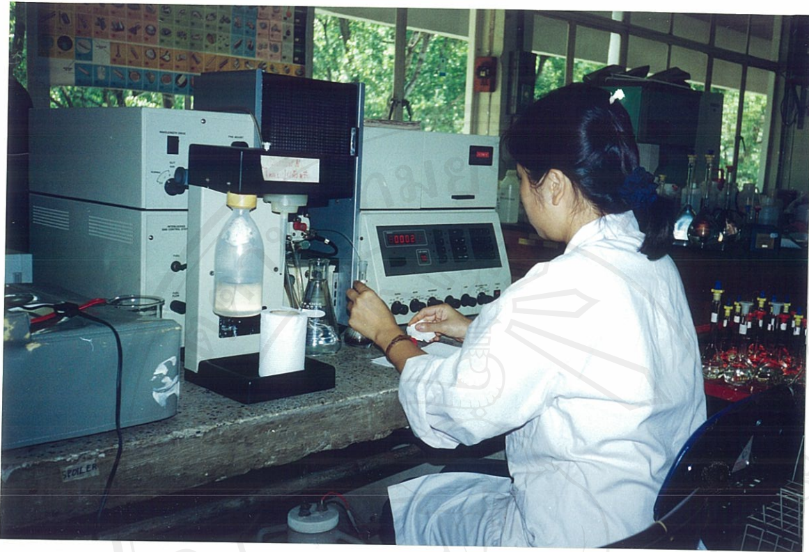
Figure 4.3. The flame AAS Perkin Elmer 2380 used in the analysis.
