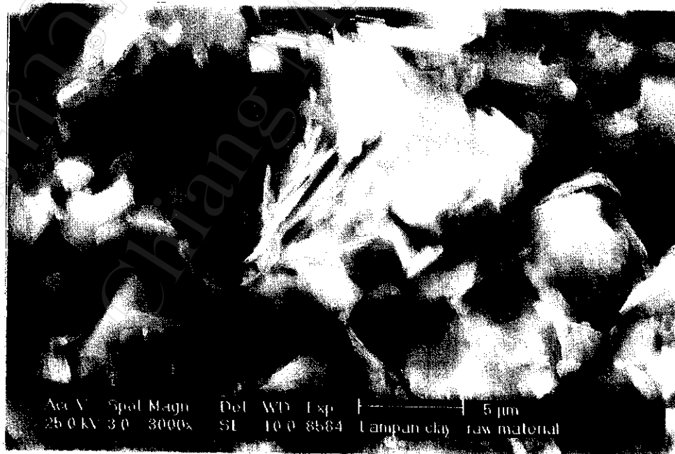
Figure 3.9 : Picture of raw Lampang clay at room temperature, 3000x magnification
