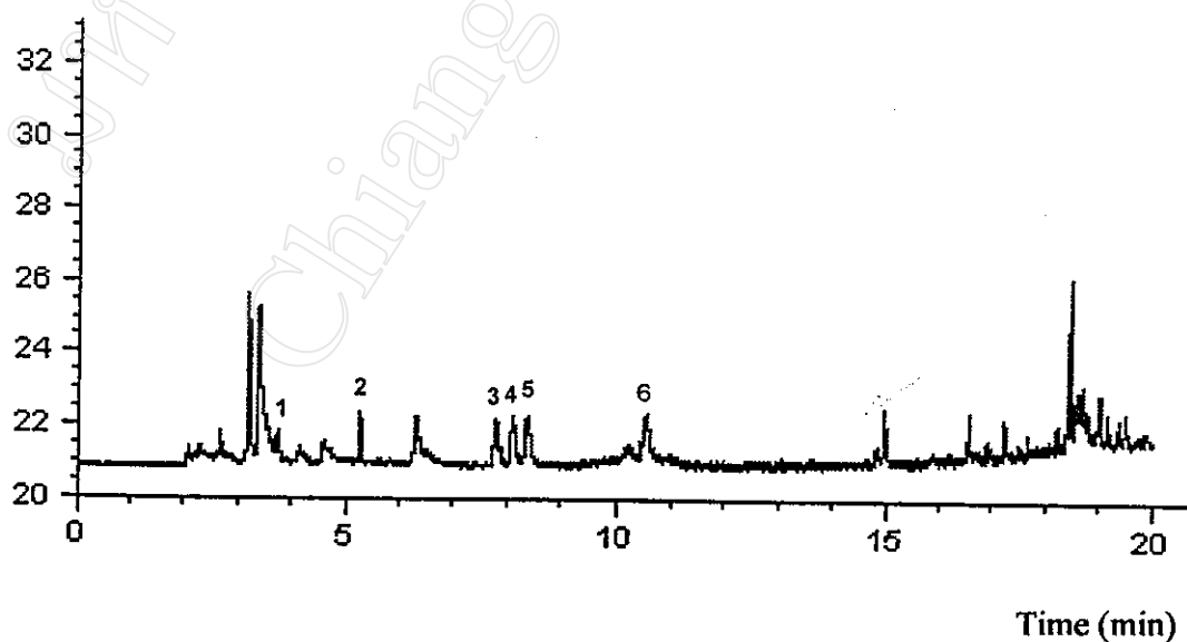
Figure 3.50 GC-FID chromatogram of 4 \mu\text{g/L} of benzene and 2 \mu\text{g/L} of toluene, ethylbenzene, p-xylene, m-xylene and o-xylene in ultrapure water. Peaks : 1 = benzene and 2-6 correspond to the numbers indicated in Figure 3.49
