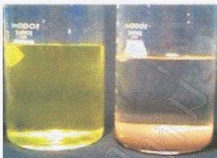
Figure 1a. Chromium Water, before/after electrocoagulation
