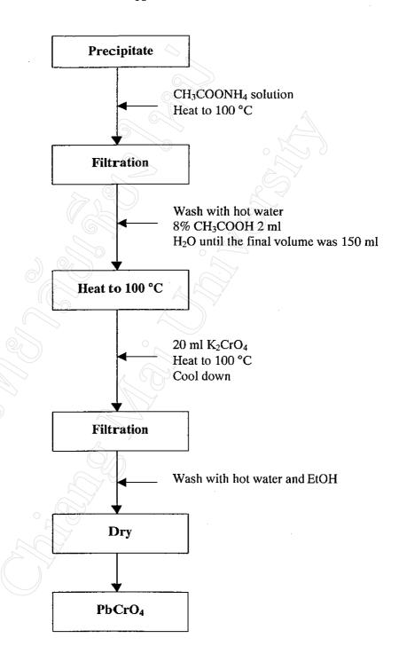
Figure 2.4 The schematic diagram of the analysis of lead as lead chromate.
