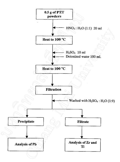
Figure 2.3 The schematic diagram for the dissolution of PZT powders.
