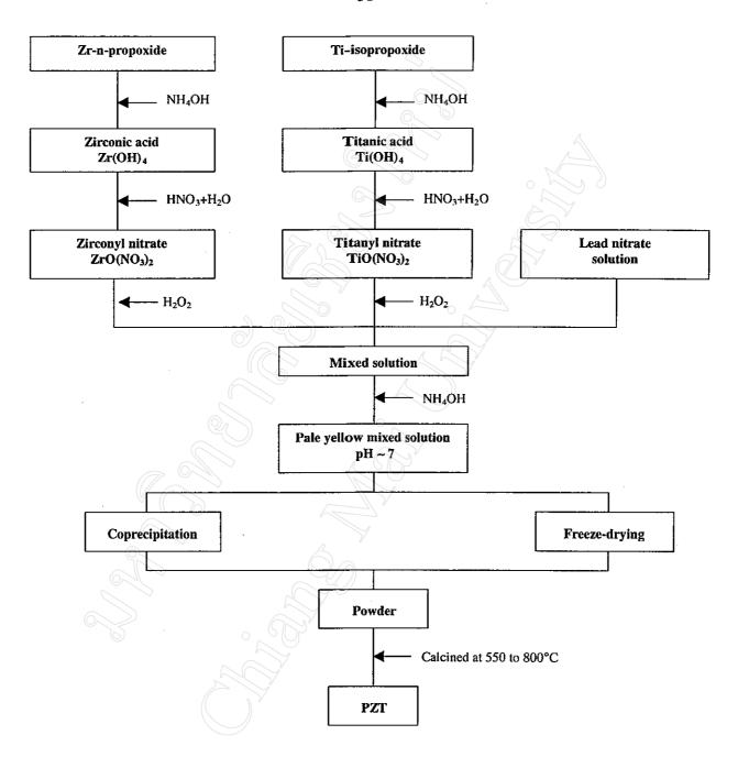
Figure 2.1 Schematic diagram for the preparation of lead zirconate titanate powders.
