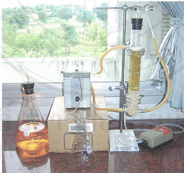
Figure 6.7 Preliminary study of continuous decolorization using packed bed bioreactor, a good decolorization efficiency could be achieved in room temperature
