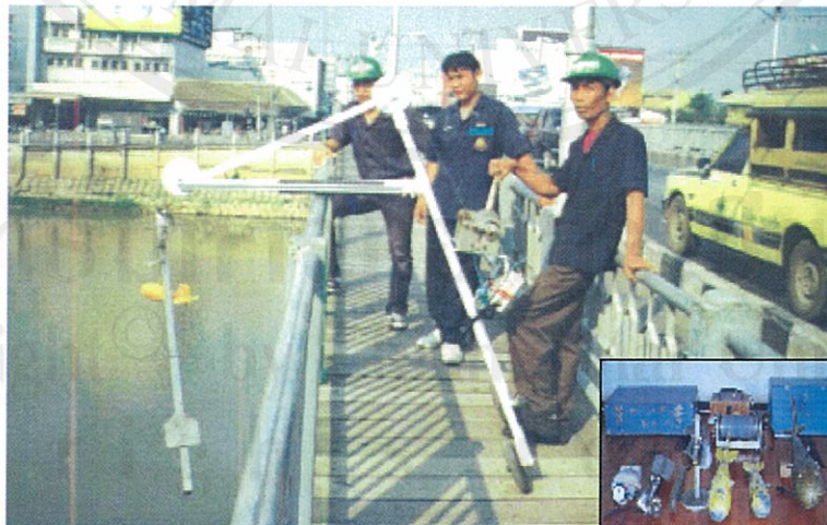
Figure 4.8 Velocity measurement of water flowing by current meter method. Components of the cup-type current meter are shown in the downright photograph. (Courtesy of Vachirasak Suraintaragoon).
