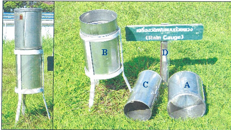
Figure 4.4 The rain gauge. A is an upper cylinder with a 8-inch diameter. Its chamber collects the rain and allows it to drain through a funnel. B is a lower cylinder. It has 8-inch diameter. C is a removable container put in the lower cylinder. D is a glass measuring cylinder.
