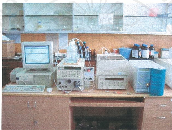
Figure 36 High performance liquid chromatograph apparatus
