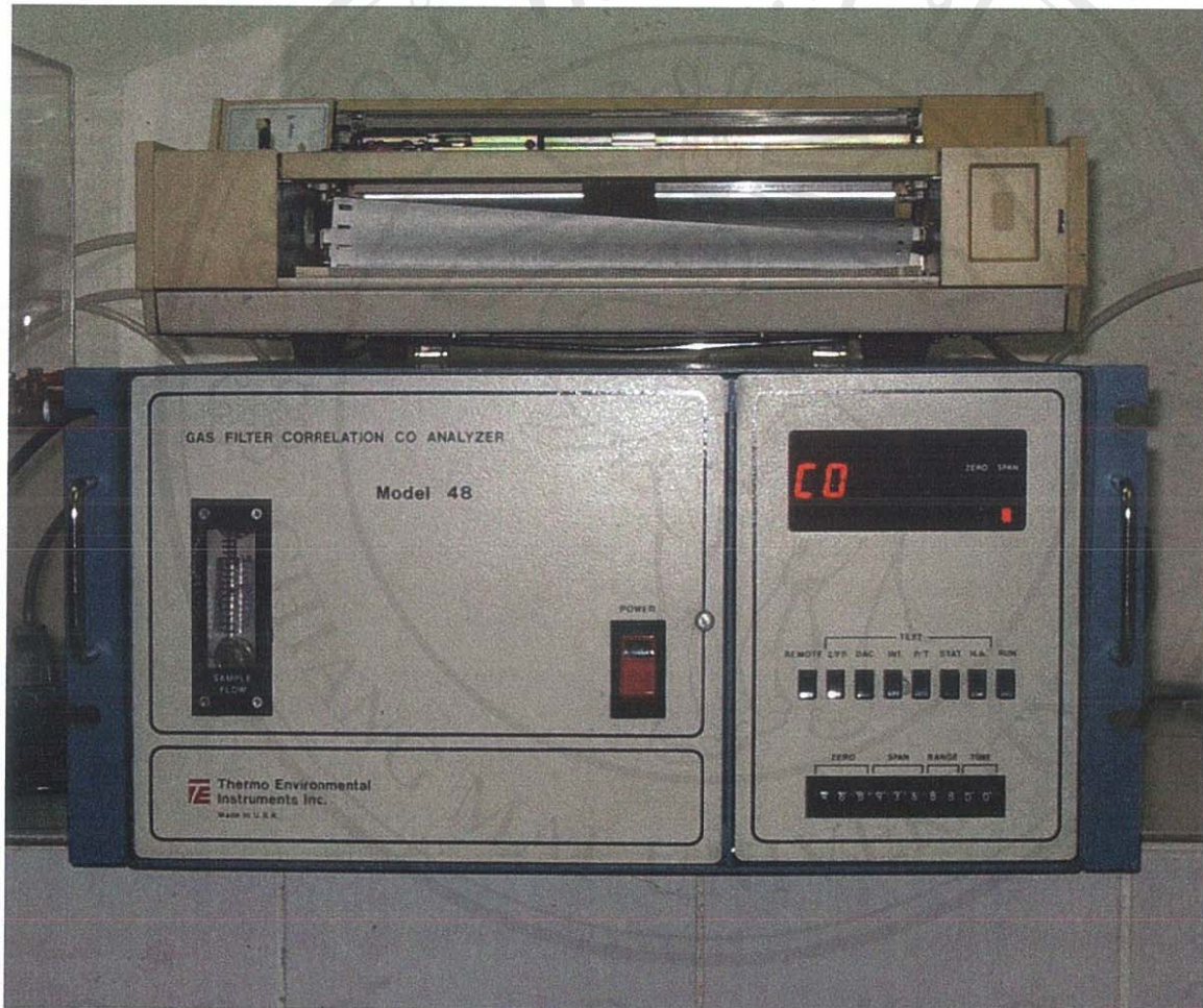
Figure 19. Gas Filter Correlation (GFC) Model 48 was used for measurement of carbon monoxide concentration in ambient air and exposure chamber.
