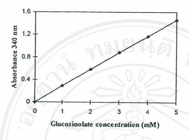
A-4 Calibration curve for the determination of sinigrin by spectrophotometric method
