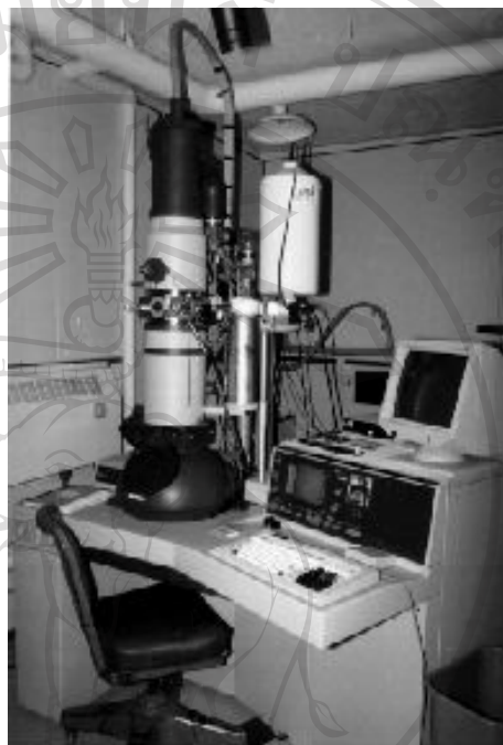
Fig. 3.9 Transmission electron microscope (TEM, Philips Tecnai 20).
