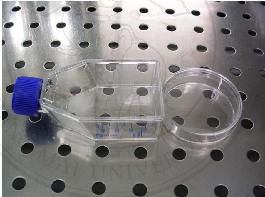
Figure 3.4 A plastic culture flask (25 cm<sup>2</sup>) and a culture dish (6 cm in diameter)
