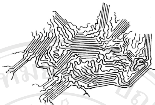
Fig. 1.6 Fringed-micelle model of the crystalline - amorphous structure of polymer [17].
