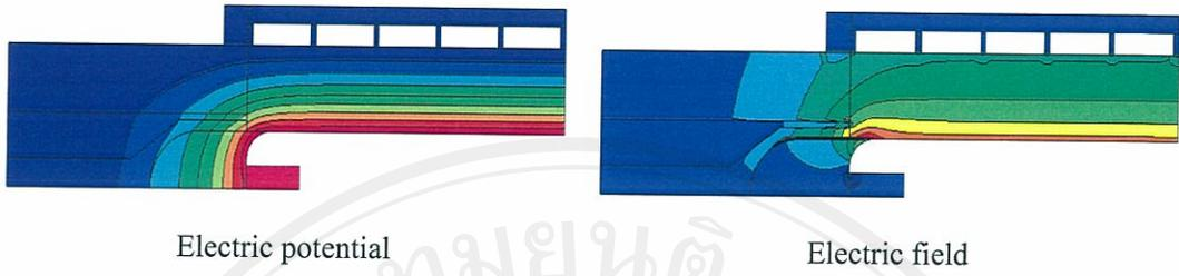
Figure 5.42 Electric potential and field plots in the classifier with flow guide as insulator, operation at 10.0 kV applied voltage.
