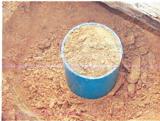
Figure 4.6 The push-core uses for collecting undisturbed samples.
