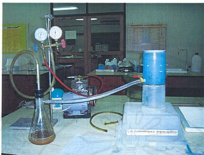
Figure 4.11 Vacuum pump attached to the resistivity box's valve as a pressure control system of the experiment.
