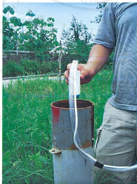
Figure 4.9 Groundwater sampling at the monitoring well.
