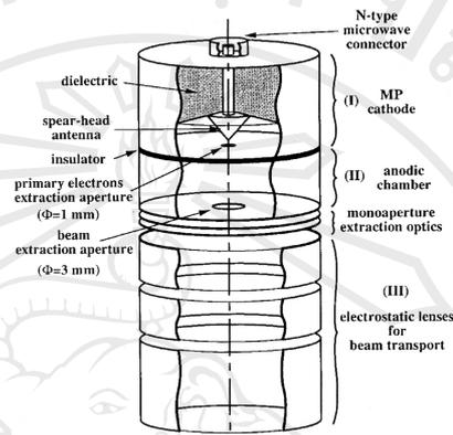
Figure 2.1. Schematic diagram of the microwave plasma cathode electron gun (Fusellier et al, 1998)
