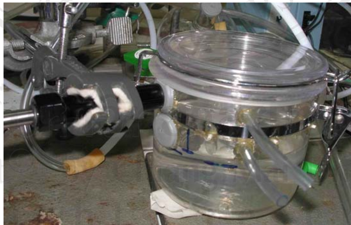
Figure 2.12 Photograph of permeation chamber while SPME sampling is being carried out in receiver chamber
