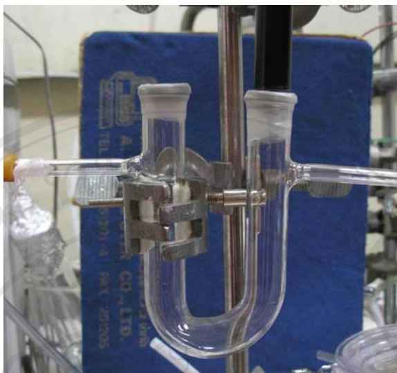
Figure 2.10 U-tube for sampling of vapor in SPME-GC calibration
