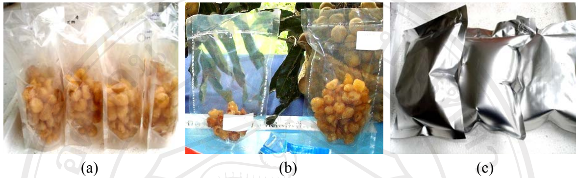
Figure 2.6 The 3 differences packaging materials in this study;(a) LLDPE material; (b) OPP material; (c) Aluminum foil material
