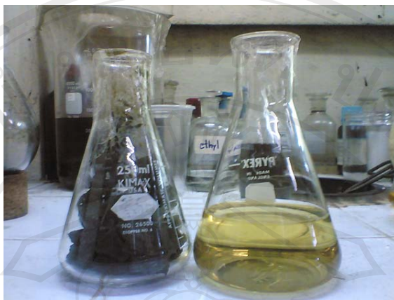
Picture 3.14 Precipitate (left) and filtrate (right) of roselle solution after electrolysis.
