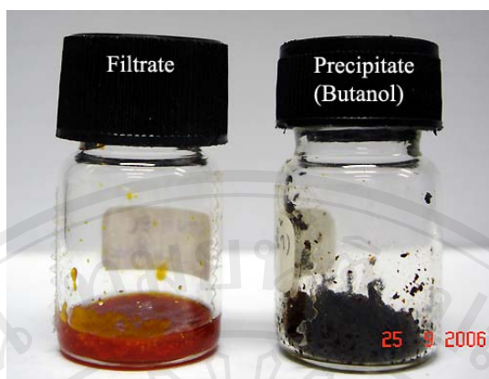
Picture 3.19 Compounds obtained from filtrate (left) and precipitate (right) after EC process of gardenia in aqueous solution (1.0 A, 40 min).
