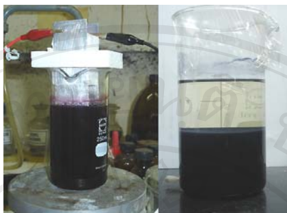
Picture 3.4 Black glutinous rice solution before (left) and after (right) electrocoagulation process.
