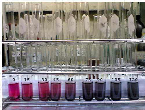
Picture 4.2 Black bean EC fractions taken every 15 min during 2 hr of EC process.
