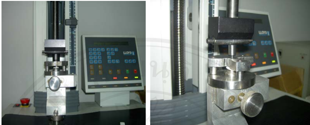
Fig. 3.3 The ball-on-ring tests
