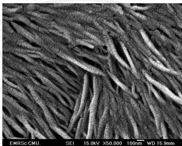
Fig. 9.2 SEM micrographs of nanoneedle-like structure of HA.
