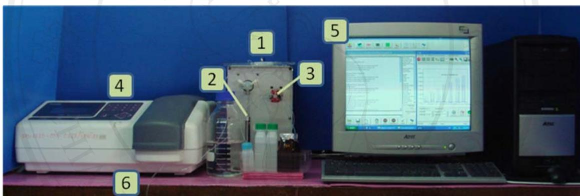
**Figure 2.3** The SIA system for determination of selenium. 1, holding coil; 2, syringe pump; 3, selection valve; 4, detector; 5, computer; 6, waste
