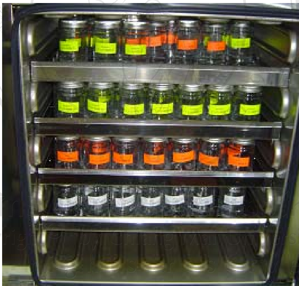
Figure 2.7 Incubator for in vitro hydrolytic degradation studies.
