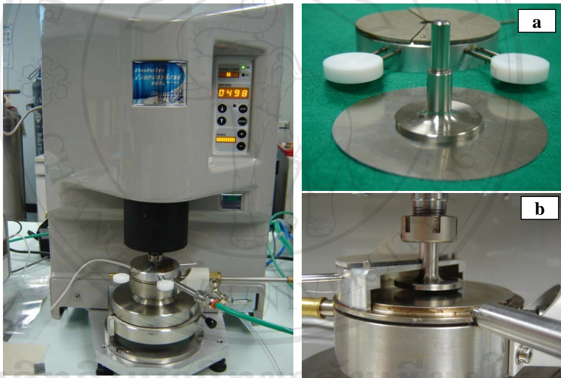
Figure 2.5 Bohlin Gemini HR nano Rotational Rheometer apparatus; (a) parallel plate geometry and (b) the gap between the plates.
