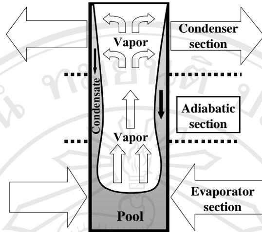
Figure 2.1 Thermosyphon (Dunn and Reay, 1982).
