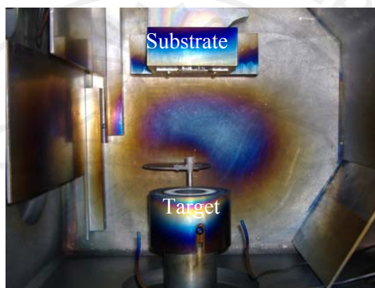
Figure 3.3 Photo of reactive magnetron sputtering setup.
