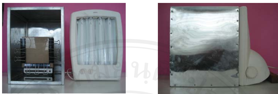
Figure 2.3. Photopolymerization apparatus with aluminium cabinet and UV-lamps.
