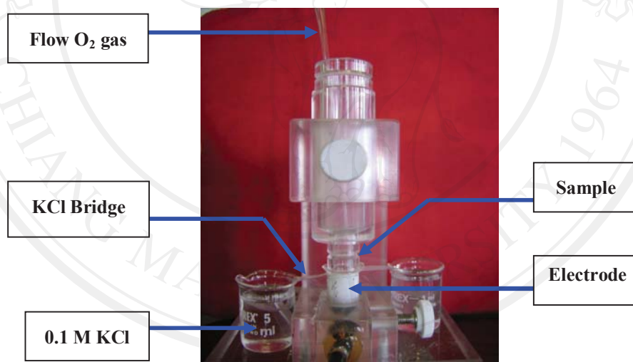
Figure 2.10. Oxygen permeability measurements were made using a 201T permimeter.
