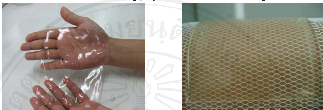
(a) without the reinforcing polymer mesh (b) with the reinforcing polymer mesh
