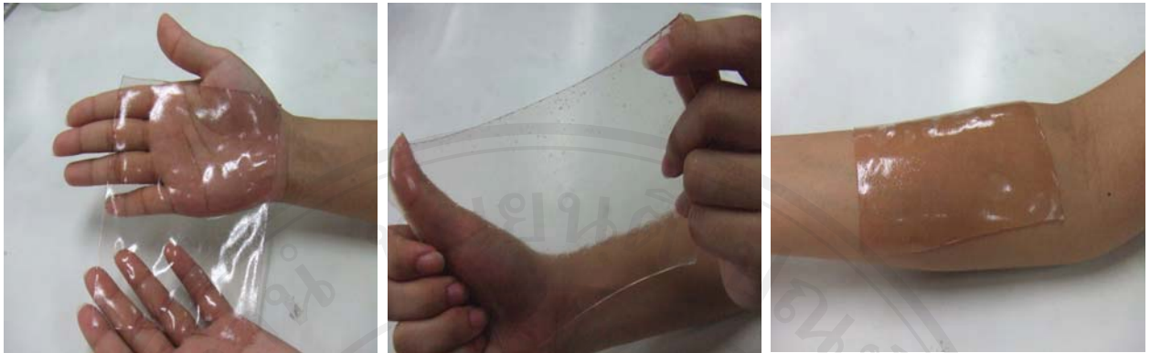
Figure 1 : Hydrogel sheets from 40% w/v Na-AMPS with 1% mol EGDM
