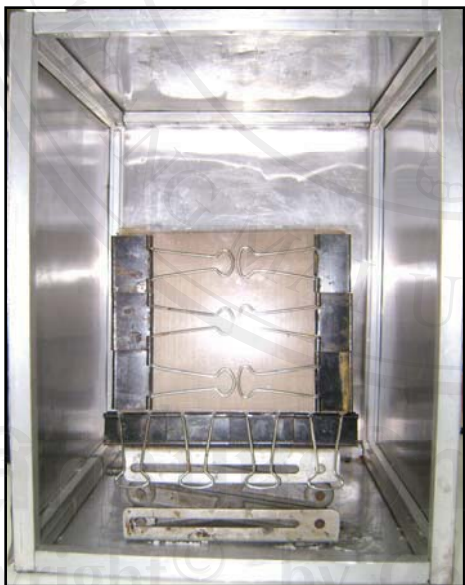
(c) Mould supported vertically on an adjustable lab jack inside the cabinet
