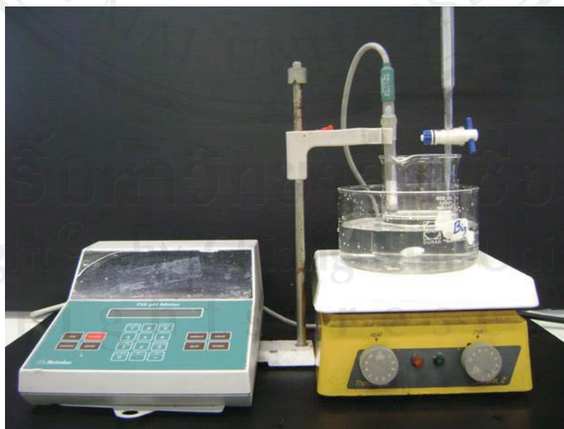
Figure 3.7: Photograph of the apparatus used in the preparation of Na-AMPS solution
