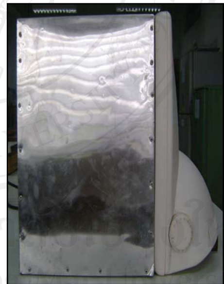
(d) UV lamp in position against the cabinet during use
