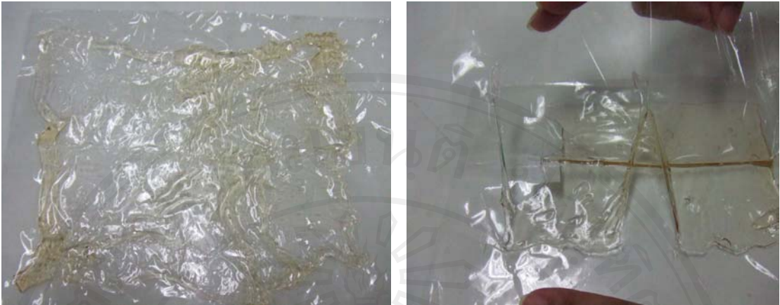
Figure 4.1 : 30% Na-AMPS hydrogel sheet (1.0% mol EGDM) prepared by redox initiation. (Thermal and photoinitiation gave similar results except that, from photoinitiation, the sheets were colourless.)
