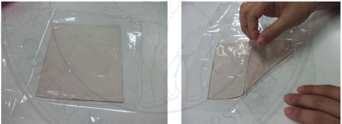
Figure 4.4 : 40% Na-AMPS hydrogel with 1% mol EGDM using redox initiation
