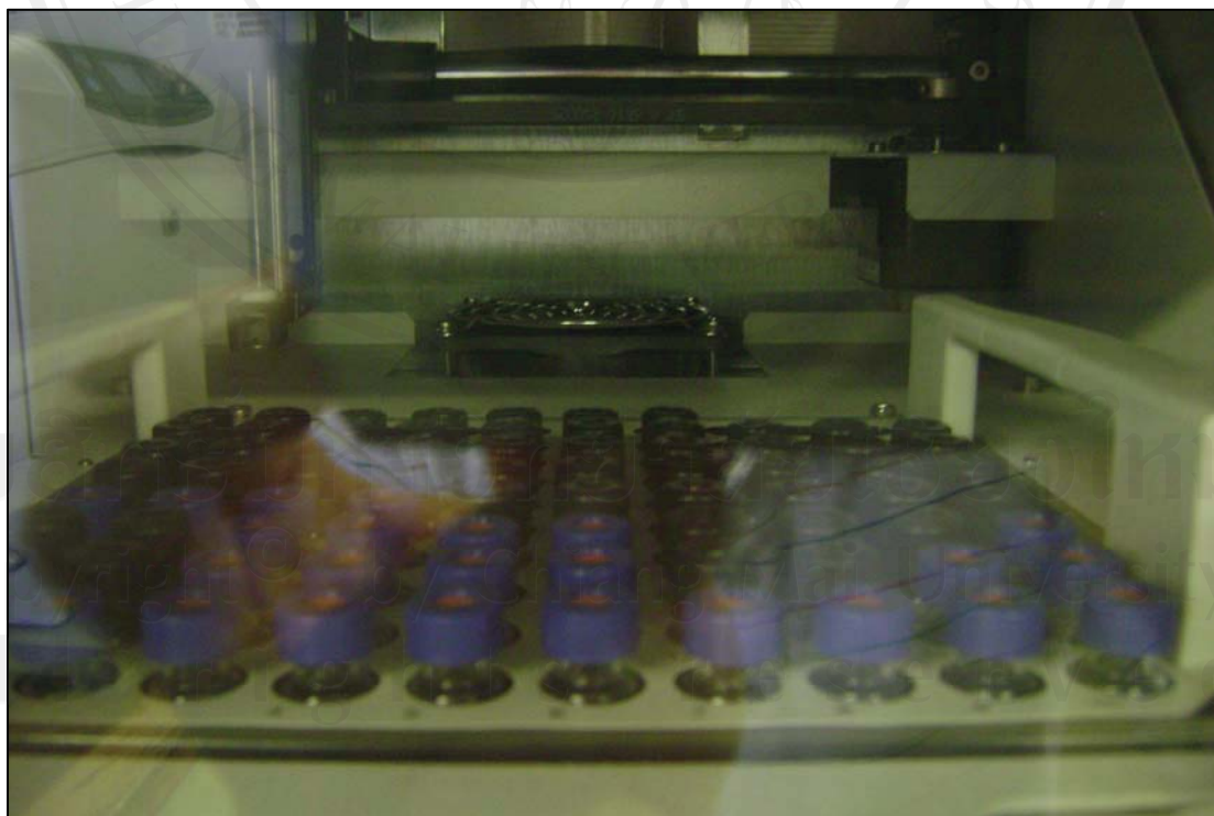
Figure 5.29: Sample arrangement in the ion chromatograph for autosampling.
