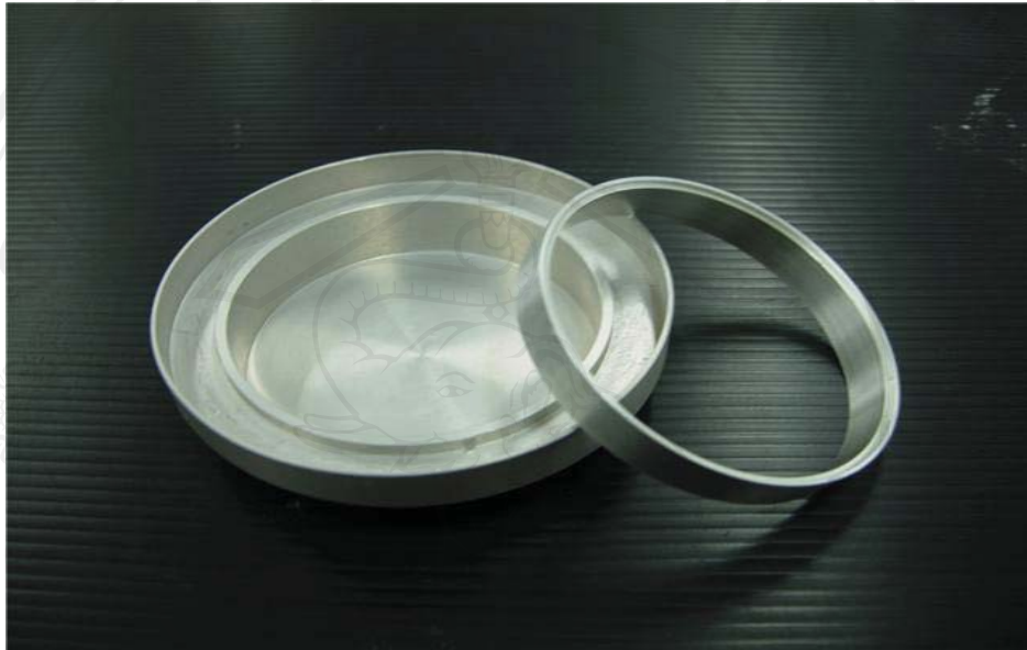
Figure 5.13 : Photograph of the water cup used for water vapour transmission rate measurements.
