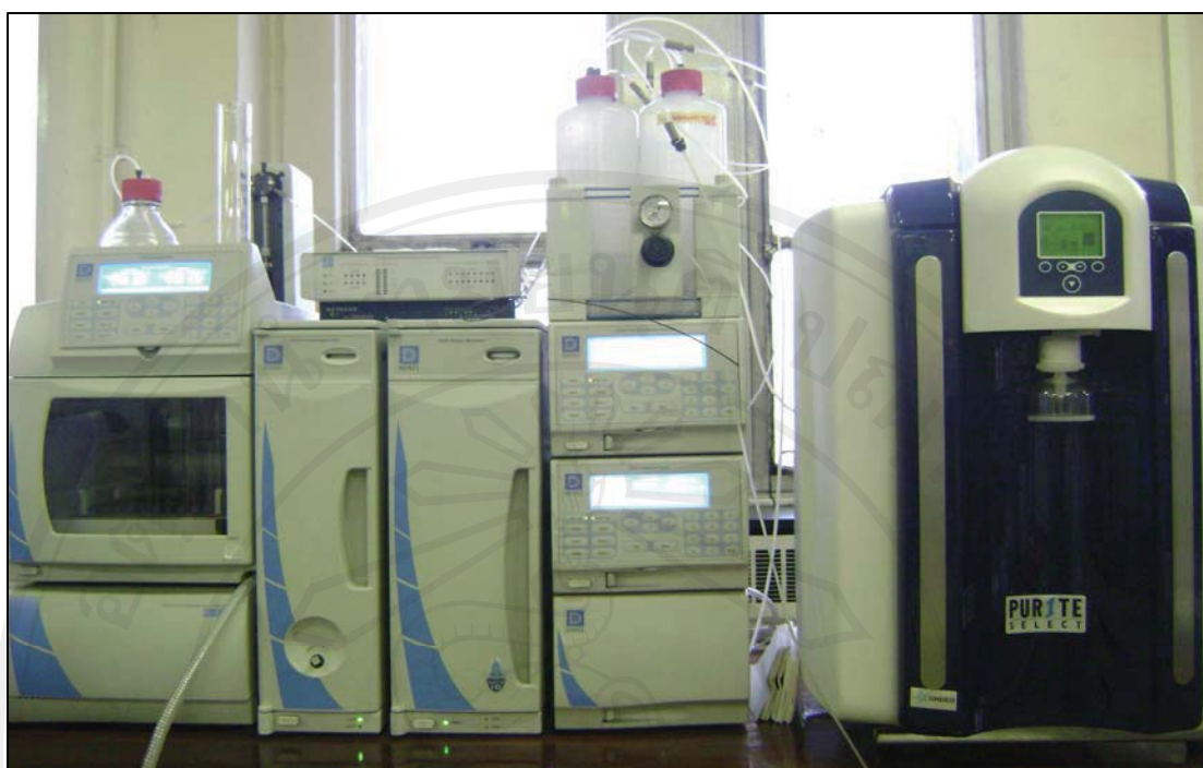
Figure 5.28 : Dionex DX600 Ion Chromatograph supported by Chromeleon Client 6.50 software used for residual monomer determination.
