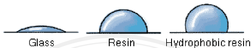
Figure 2.9 Shape of water drops on the surface of glass, resin and hydrophobic resin [27].
