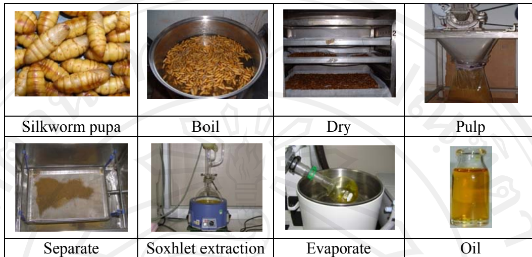
Figure 19 Extraction processes of the native Thai silkworm pupa oil by Soxhlet extraction
