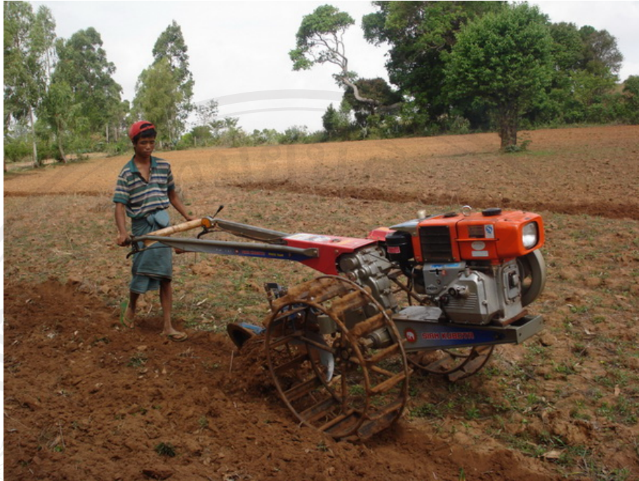
Figure 3.13: Plowing with a Power Tiller
