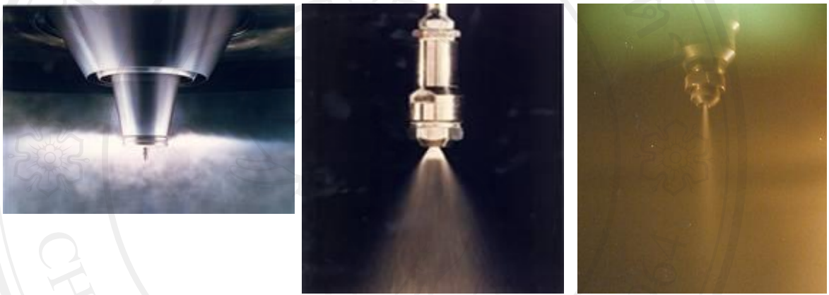
(A) Rotary atomizer
