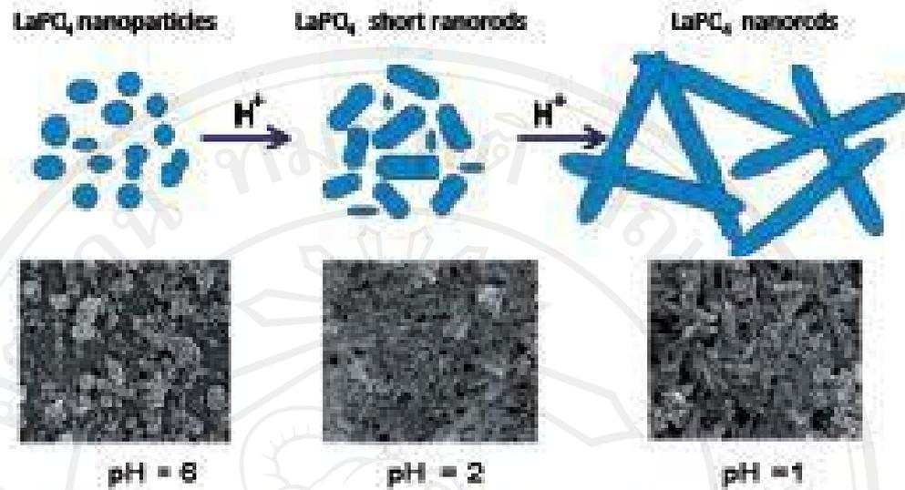
Figure 4. Schematic diagram for the formation of  $\text{LaPO}_4$  products.
