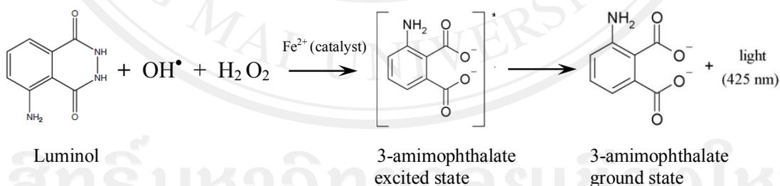
**Figure 3.1** Scheme of the suggested CL reaction mechanism
