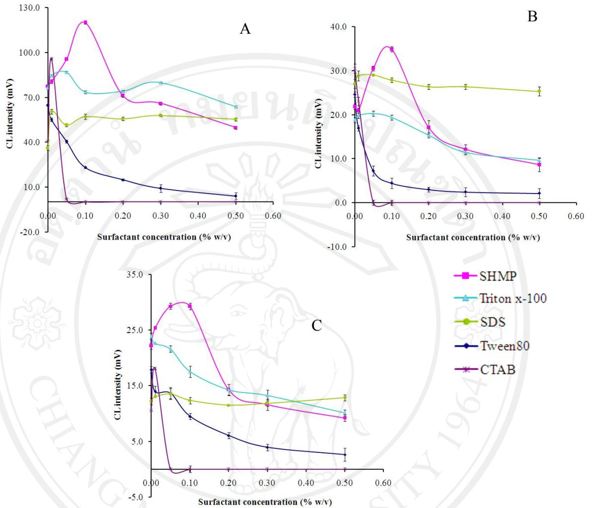
**Figure 3.5** Effect of surfactant variables on CL intensity of NFZ (A), NFT (B) and
