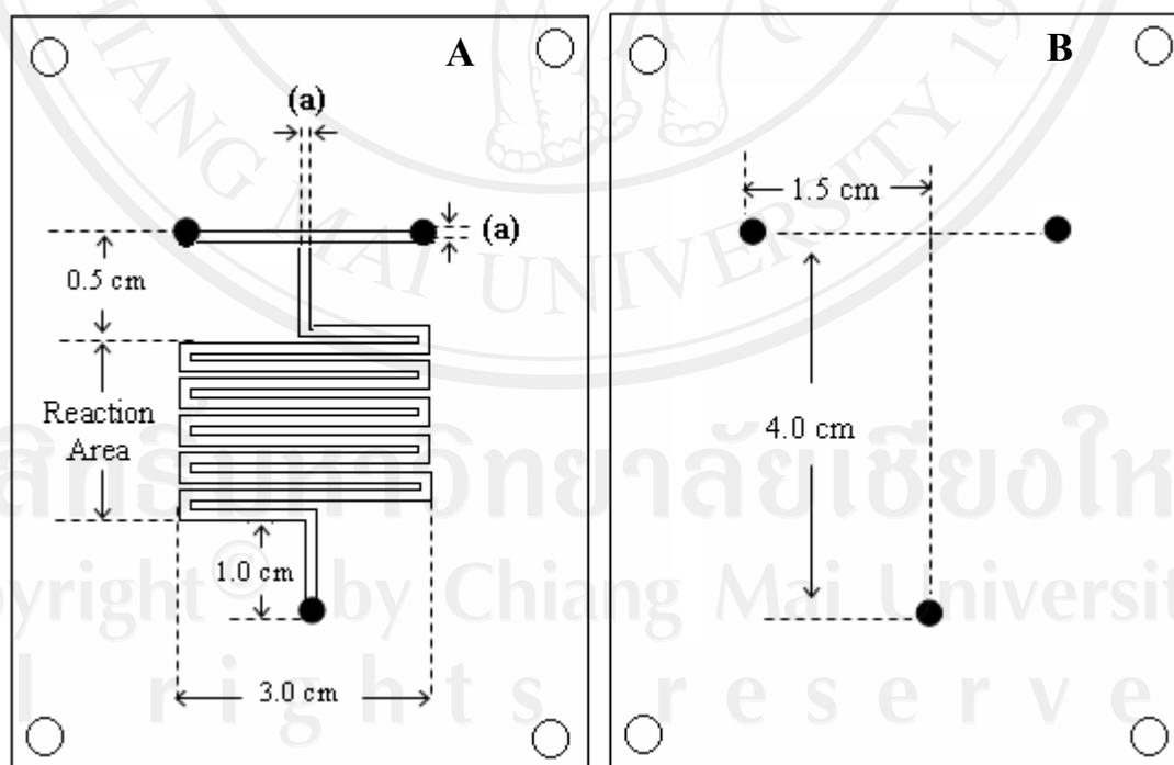
**Figure 3.3** The dimensions of the microchannels on the microfluidic device. Base plate (A); Top plate (B)
