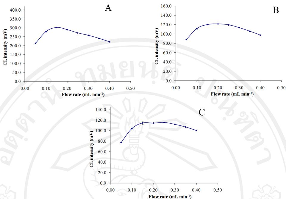
**Figure 3.14** Effect of flow rate of a oxidant/surfactant stream on the CL intensity for the determination of NFZ (A), NFT (B) and FZD (C)
