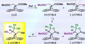
Scheme 1. Synthesis of TADDOL-anthracene adduct (11 R )-1. Reagents and conditions: (i) a. 1.2 equiv LDA, THF, -78 °C to 0 °C, 2 h, b. 1.2 equiv benzophenone, 0 °C to rt, 2 h (ii) 20 equiv LiAlH 4 , THF -78 °C to rt, 3 days
