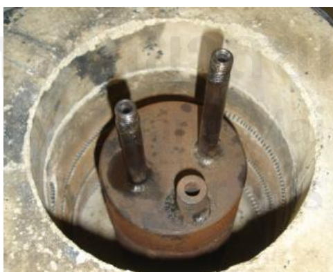
The High Pressure Vessel Placed Inside the Oven
