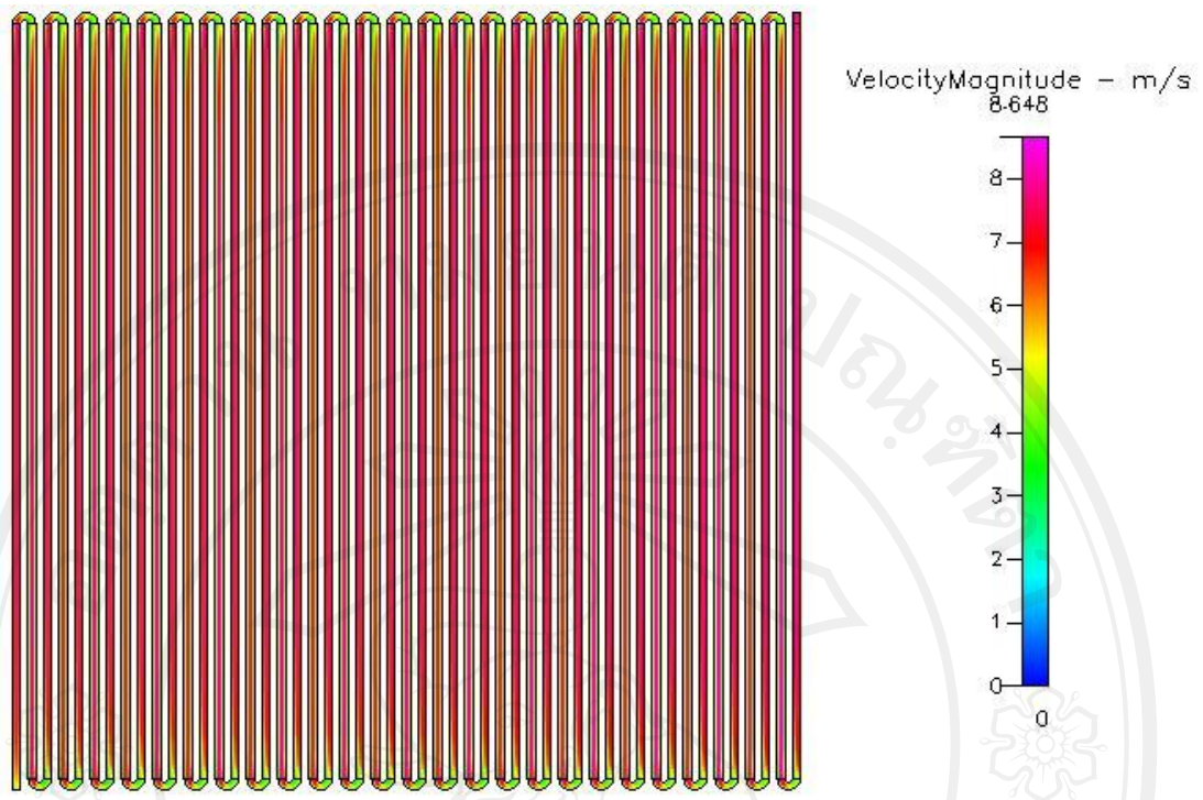
Figure 5.9 Velocity distribution at 300 cm 3 /min of fillet curve
