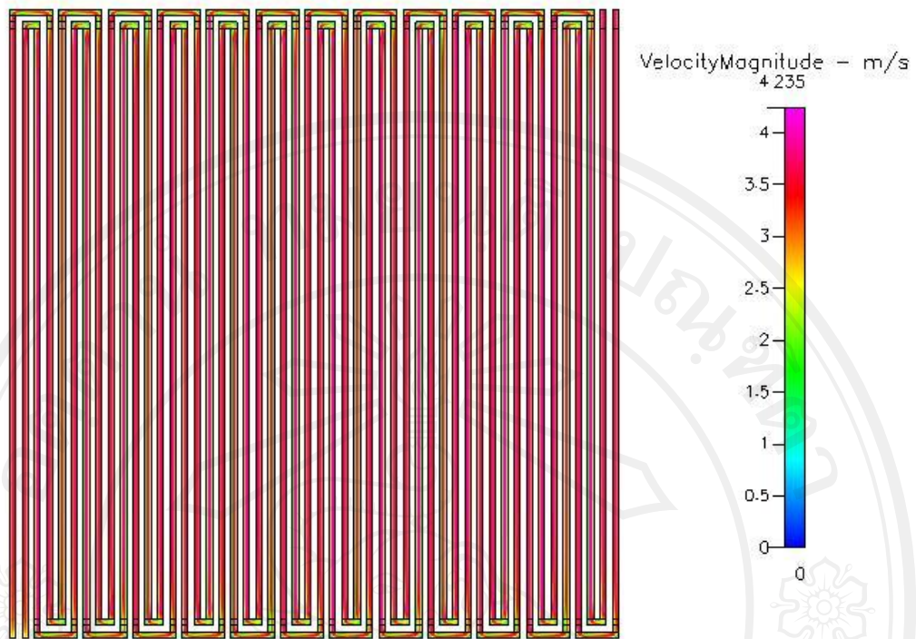
Figure 5.20 Velocity distribution at 300 \text{ cm}^3/\text{min} of 2 channels
