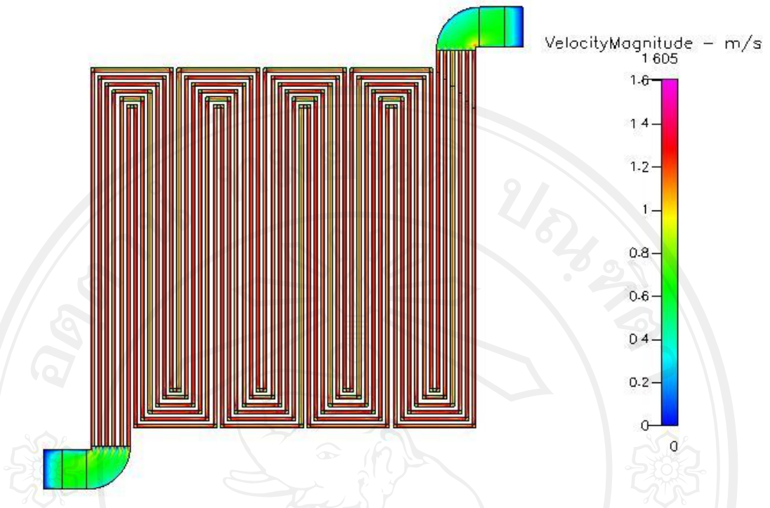
Figure 5.69 Velocity distribution at 300 \text{ cm}^3/\text{min} of type 2 manifold
