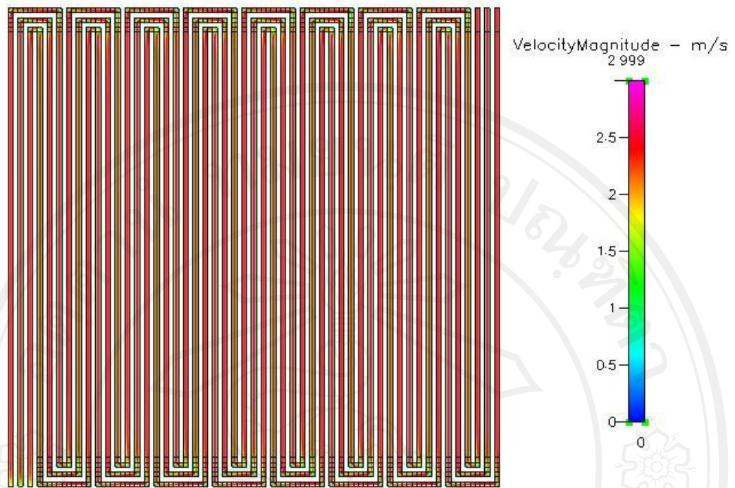
Figure 5.22 Velocity distribution at 300 \text{ cm}^3/\text{min} of 3 channels
