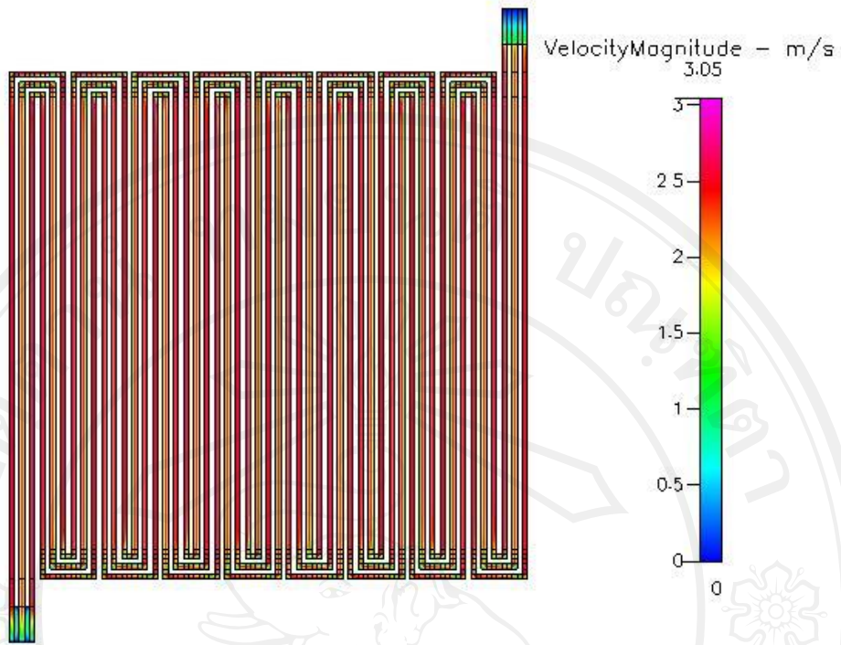
Figure 5.50 Velocity distribution at 300 \text{ cm}^3/\text{min} of manifold 3 channels
