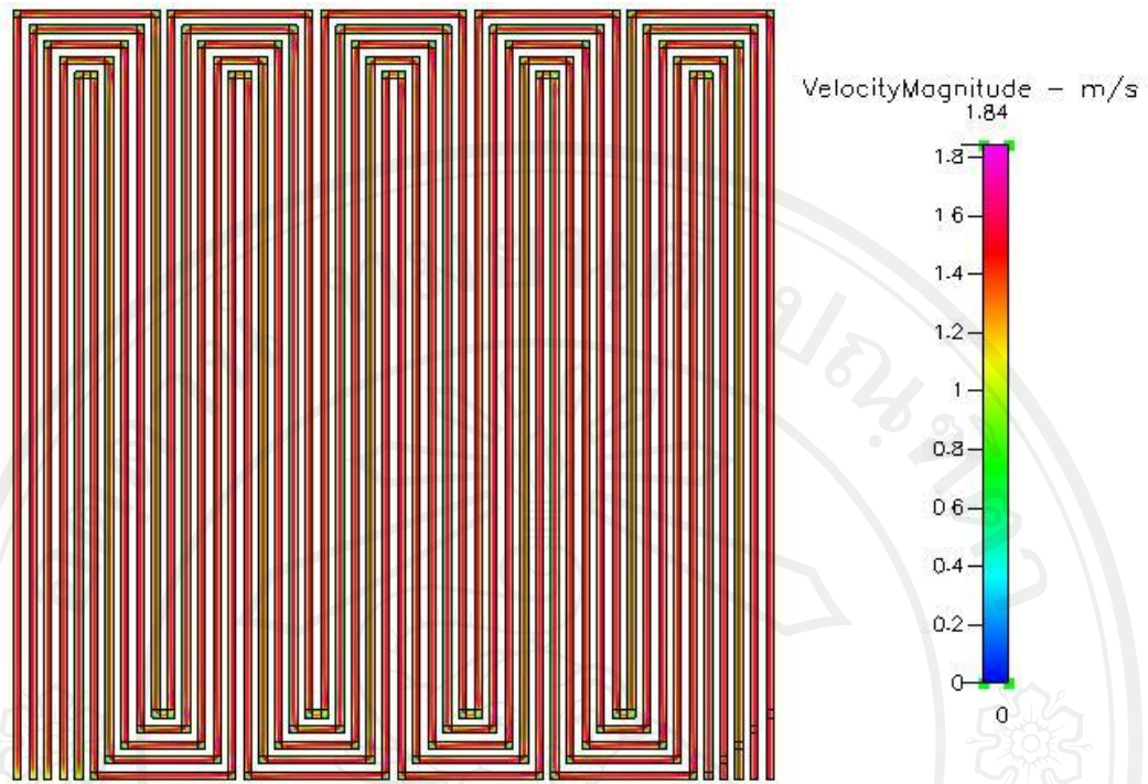
Figure 5.26 Velocity distribution at 300 \text{ cm}^3/\text{min} of 5 channels
