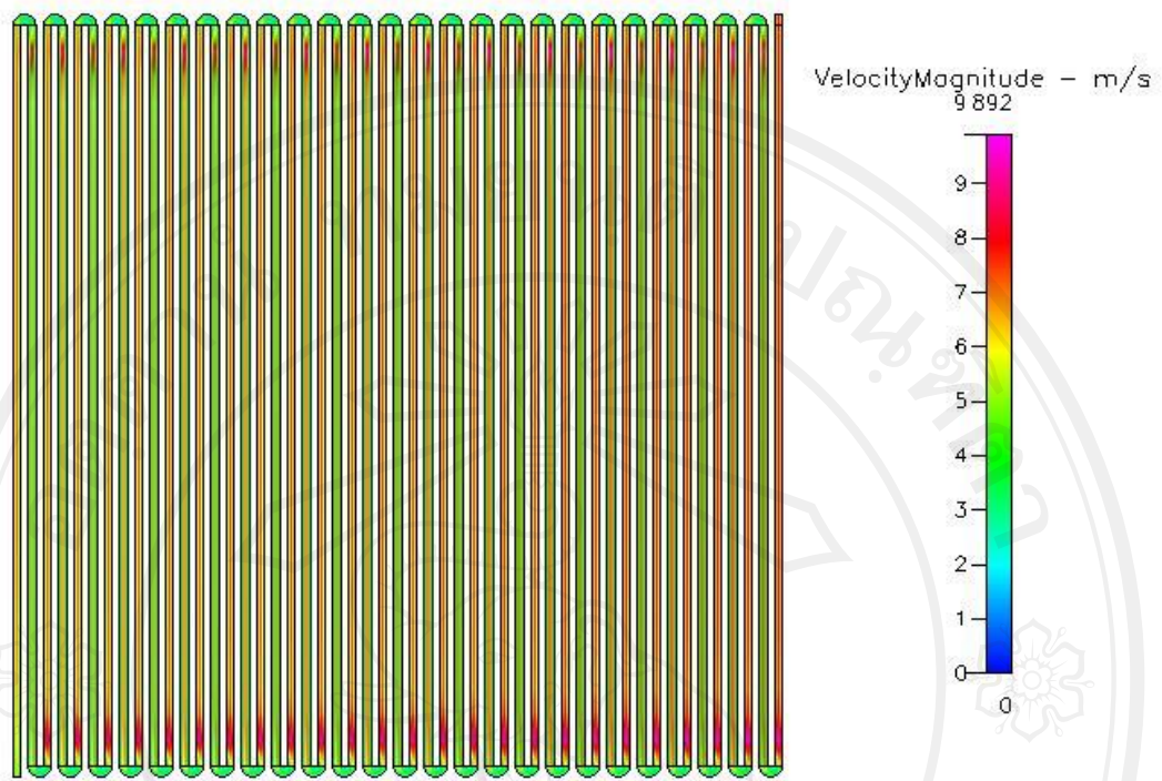
Figure 5.7 Velocity distribution at 300 \text{ cm}^3/\text{min} of outside fillet curve
