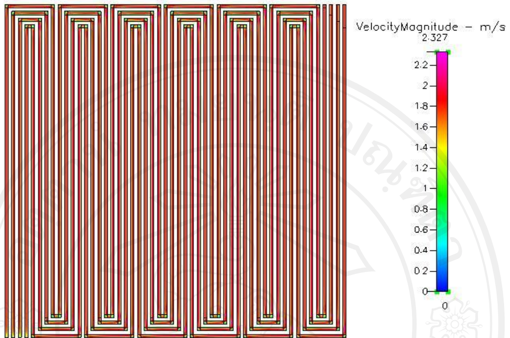
Figure 5.24 Velocity distribution at 300 \text{ cm}^3/\text{min} of 4 channels
