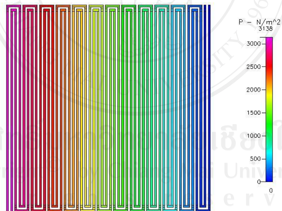
Figure 5.21 Pressure distribution at 300 \text{ cm}^3/\text{min} of 2 channels
