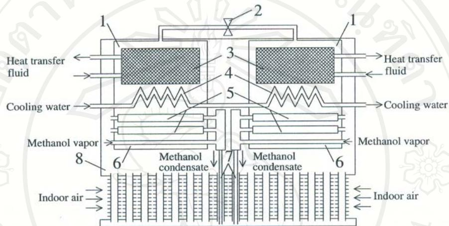
Figure 1.4 Schematic diagram of the compact adsorption room air conditioner.
