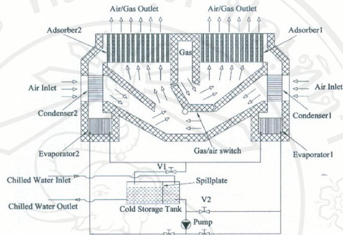
Figure 1.7 Schematic diagram of the air conditioner in the locomotive operator cabin (Wang et al., 2006b).
