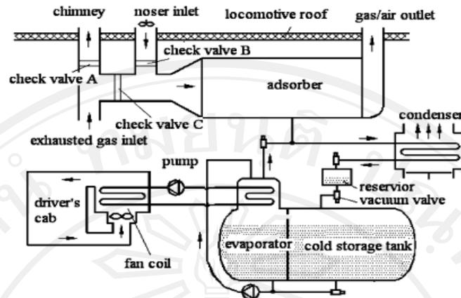
Figure 1.2 Schematic diagram of the adsorption air conditioner installed in the locomotive (Lu et al., 2004).
