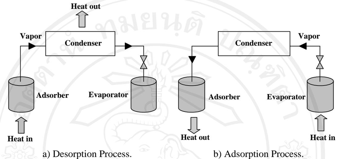
Figure 2.1 Basic operating principle of adsorption process.
