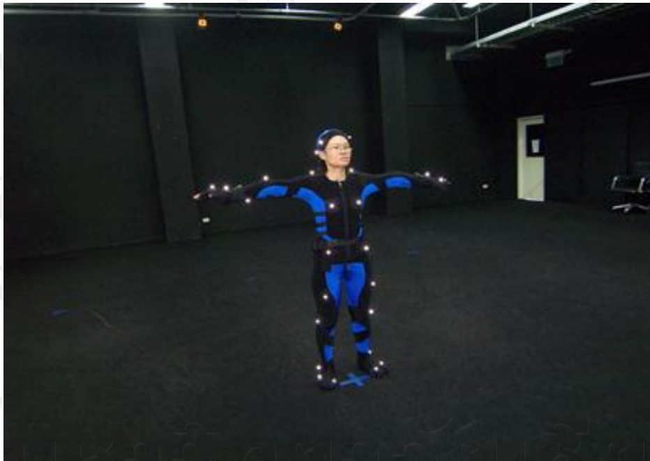
Figure 4.7 The motion capture suit, body and glove marker setting in the sign language model (Sign language model)
