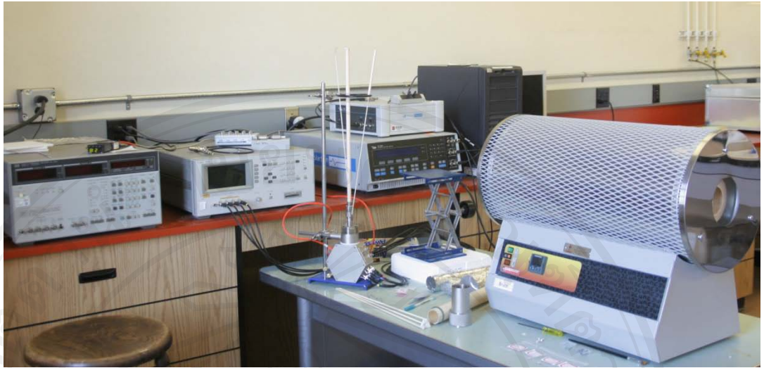
Figure 3.7 Photo images of the dielectric (Agilent 4284A LCR meter) and electrical measurement system (HP 4194A impedance analyzer)
