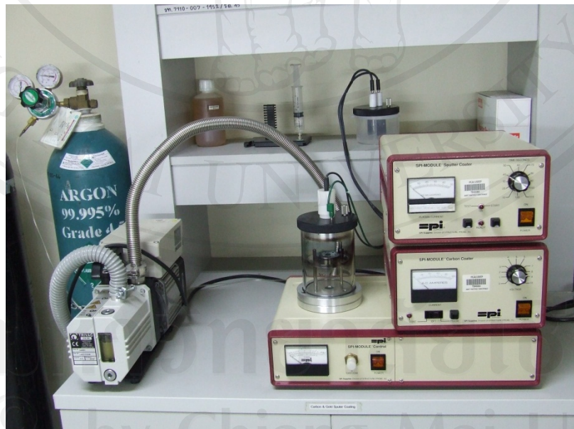
Figure 3.13 Sputter coater (JFC-1100E).
