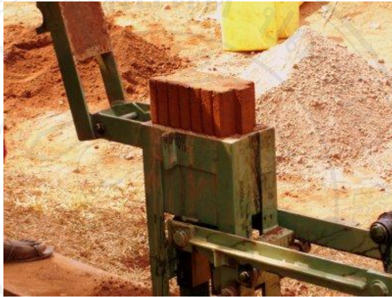
Figure. 2.2 Dry press process for making clay bricks [21].
