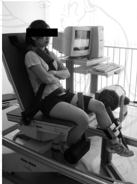
Figure 7 Measurement of quadriceps muscle strength by use isokinetic dynamometer
