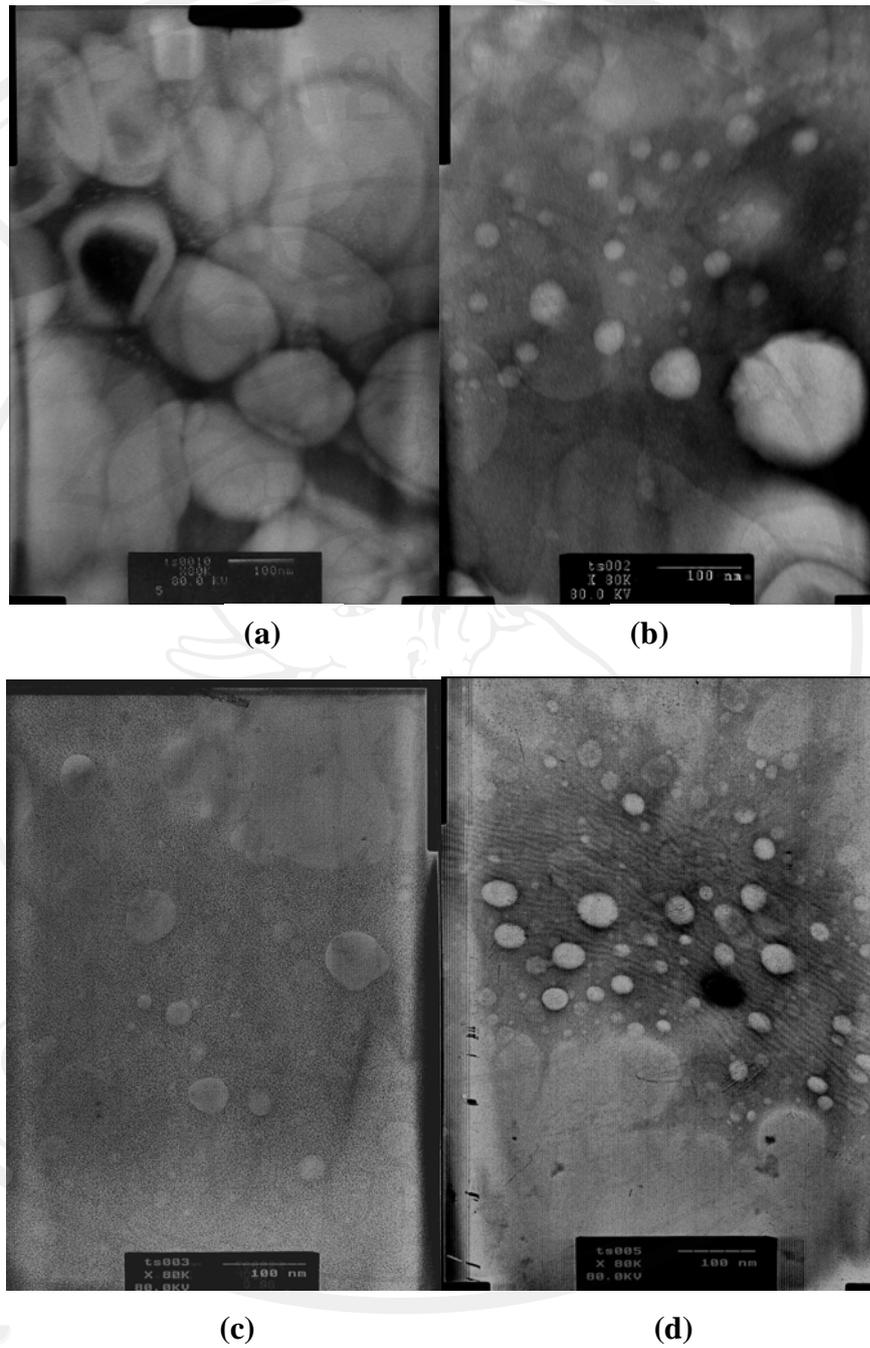
**Figure 34** Negative staining TEM images of conventional niosomes and elastic niosomes loaded with DCFD. (a) conventional Tween61 niosomes ( $\times 80K$ ). (b) elastic Tween61 niosomes ( $\times 80K$ ). (c) conventional Tween61 niosomes loaded with DCFD ( $\times 80K$ ). (d) elastic Tween 61 niosomes loaded with DCFD ( $\times 150K$ ).
